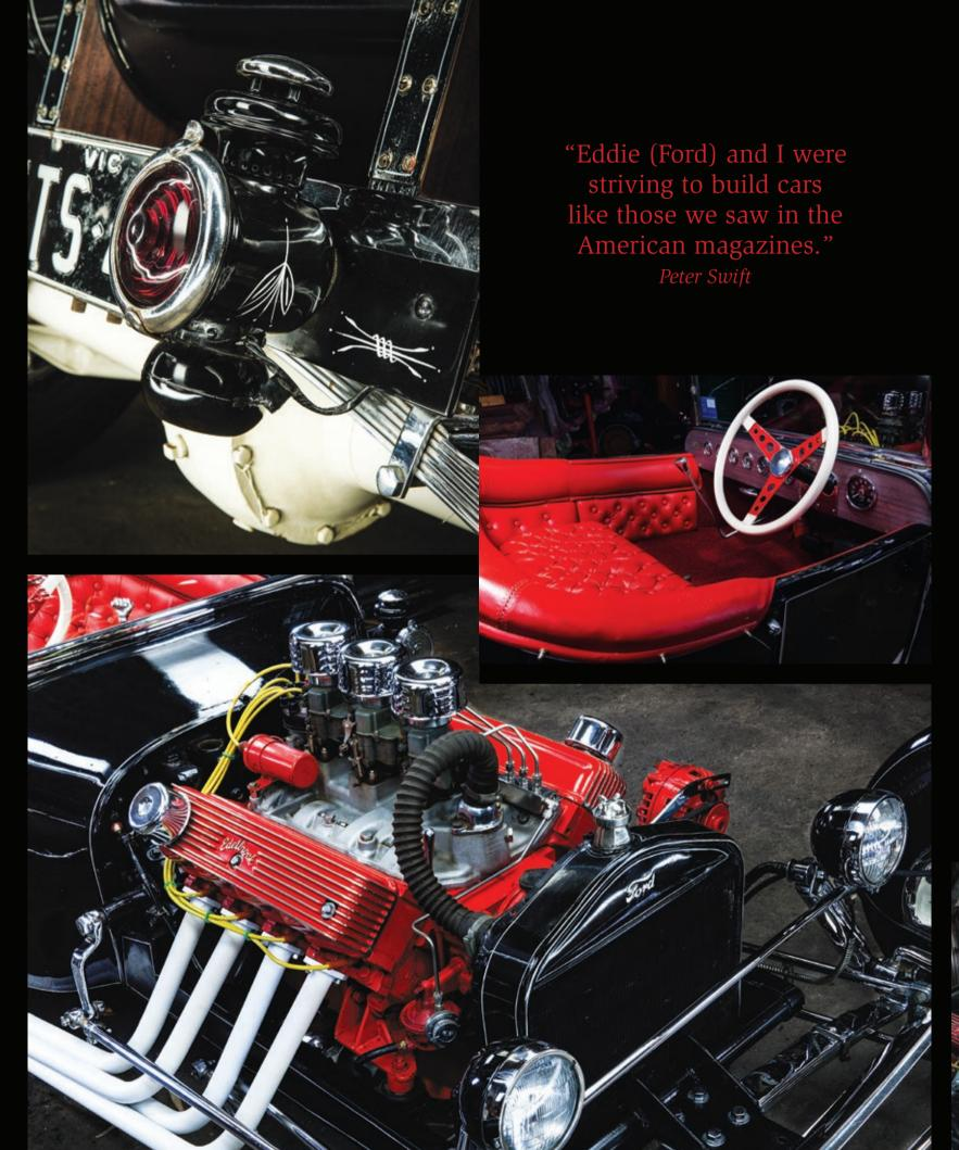
When he did return home he brought with him an intake manifold Phil Weiand had given to him, an Autolite four-barrel carburettor, Cal Custom scoop, and a W&H Du-Coil dual-coil distributor he also got from Weiand.
